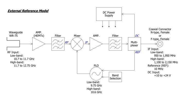
Fig.2 Functional Block Diagram
